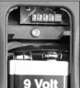
Figure 13: DIP Switch in Remote Handset Battery Compartment.
